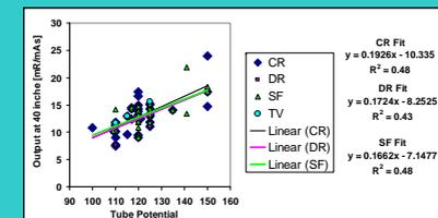
Figure 5 – X-ray tube outputs stratified by receptor design
